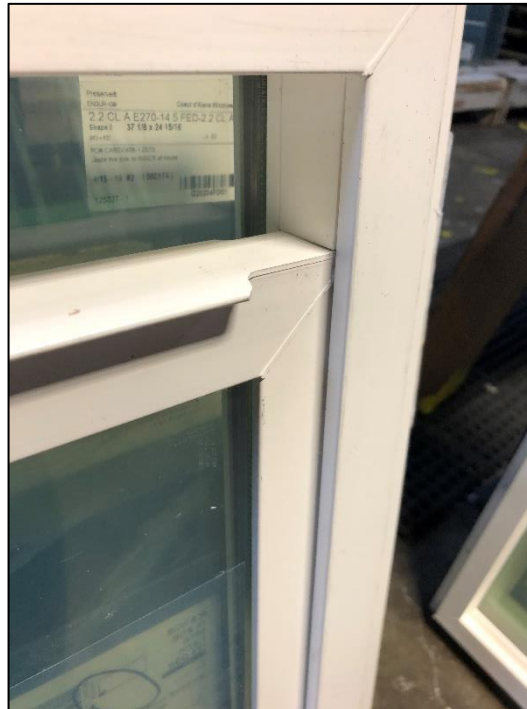
Sash inserted, ready to close
