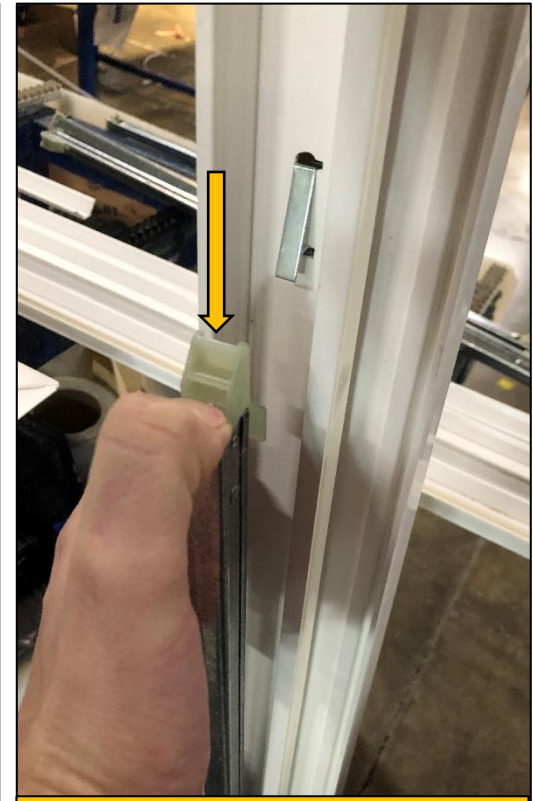
Push down on balancer (#2)
